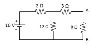
3. (a) Determine the mesh currents for the circuit shown below. [L4][5M]
